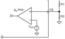
Figure 7. Voltage-Divider Configuration
