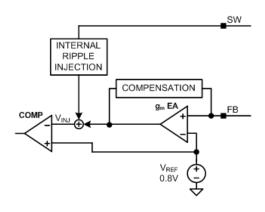
Figure 8. Internal Ripple Injection
