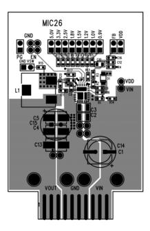
Figure 10. MIC26903 Evaluation Board Top Layer
