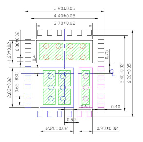
Red circle indicates Thermal Via. Size should be .300-.350 mm in diameter, 0.80 mm pitch, and it should be connected to GND plane for maximum thermal performance.
