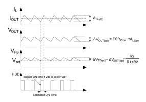
Figure 2. MIC26903 Control Loop Timing
