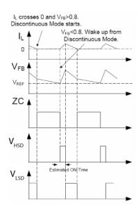
Figure 4. MIC26903 Control Loop Timing (Discontinuous Mode)
