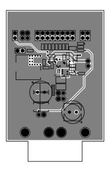
Figure 12. MIC26903 Evaluation Board Mid-Layer 2
