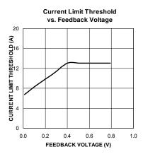
Figure 5. MIC26903 Current Limit Foldback Characteristic
