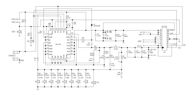
Figure 9. Schematic of MIC26903 Evaluation Board (J11, R13, R15 are for testing purposes)
