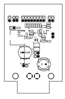
Figure 11. MIC26903 Evaluation Board Mid-Layer 1 (Ground Plane)
