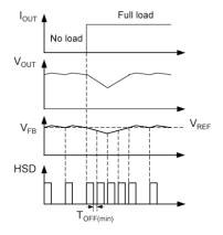
Figure 3. MIC26903 Load Transient Response
