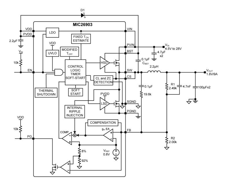
Figure 1. MIC26903 Block Diagram
