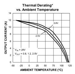
**Die Temperature\***: The temperature measurement was taken at the hottest point on the MIC26903 case mounted on a 5 square inch 4 layer, 0.62", FR-4 PCB with 2oz finish copper weight per layer, see Thermal Measurement section. Actual results will depend upon the size of the PCB, ambient temperature and proximity to other heat emitting components.
