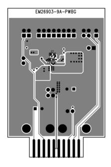
Figure 13. MIC26903 Evaluation Board Bottom Layer
