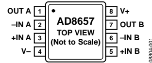
Figure 1. AD8657 Pin Configuration, 8-Lead MSOP
