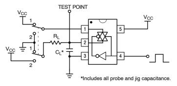
Figure 8. Propagation Delay Output Enable/Disable
