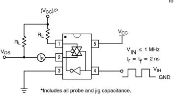
Figure 12. Feedthrough Noise, ON/OFF Control to Analog Out, Test Set-Up
