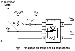
Figure 13. Total Harmonic Distortion Test Set-Up
