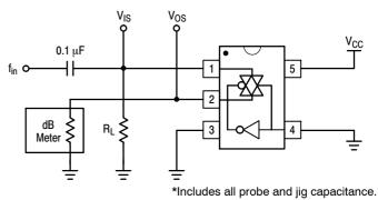
Figure 11. Off-Channel Feedthrough Isolation
