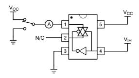
Figure 6. Maximum On-Channel Leakage Current Test Set-Up
