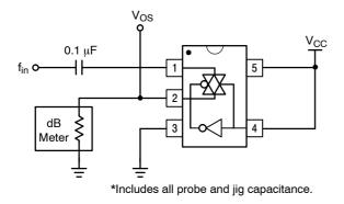
Figure 10. Maximum On-Channel Bandwidth
