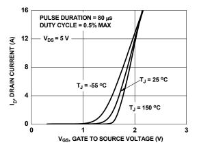
Figure 5. Transfer Characteristics
