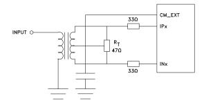
Figure 6: Transformer coupled input
