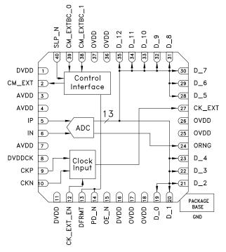
Figure 1. Functional Block Diagram
