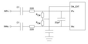
Figure 7: AC coupled input
