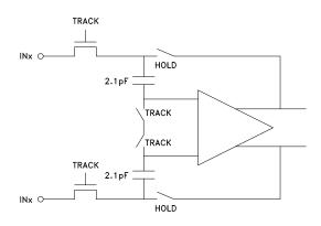
Figure 4: Input configuration
