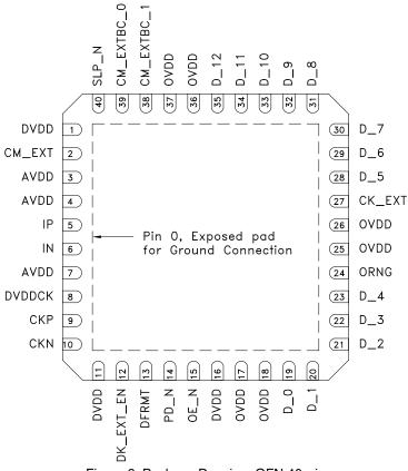
Figure 3: Package Drawing, QFN 40-pin
