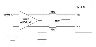
Figure 5: DC coupled input with buffer
