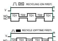
V = Voltage NO = Normally Open Contact NC = Normally Closed Contact TD1, TD2 = Time Delay R = Reset
