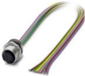
Sensor/actuator flush-type socket, 12-pos., M12 SPEEDCON, front/screw mounting with M16 thread, with 0.5 m PVC litz wire, 12 x 0.14 mm
