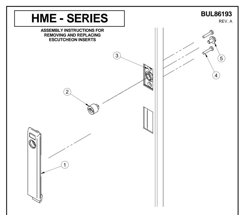
A) Open door and make sure ratchet gear (item 3) is either fully extended or fully retracted by turning the insert fully left or right.
