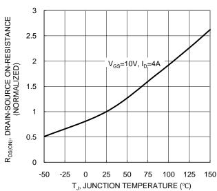
Figure 6. On-Resistance Variation with Temperature
