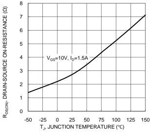
Figure 7. On-Resistance Variation with Temperature
