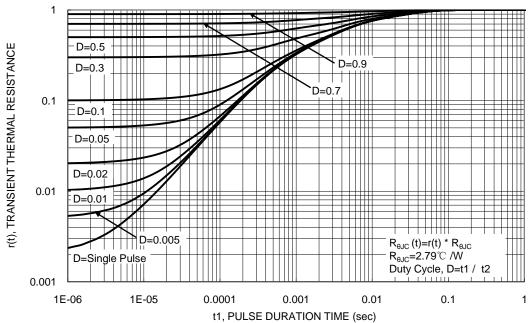
Figure 13. Transient Thermal Resistance
