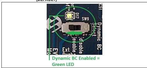
FIGURE 2-9: DYNAMIC BATTERY CHARGE SELECT DISABLED
