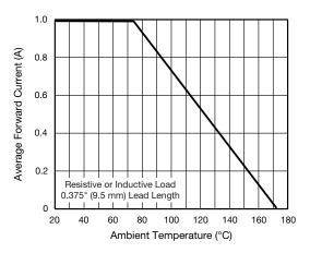
Fig. 1 - Forward Current Derating Curve
