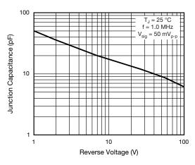
Fig. 5 - Typical Junction Capacitance
