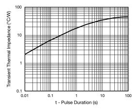
Fig. 6 - Typical Transient Thermal Impedance
