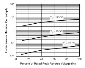
Fig. 4 - Typical Reverse Characteristics
