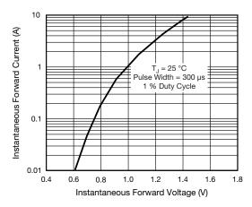
Fig. 3 - Typical Instantaneous Forward Characteristics
