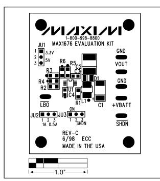
Figure 2. MAX1676 EV Kit Component Placement Guide— Component Side
