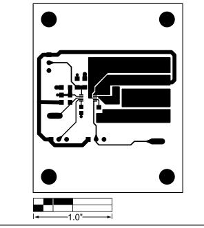
Figure 3. MAX1676 EV Kit PC Board Layout—Component Side
