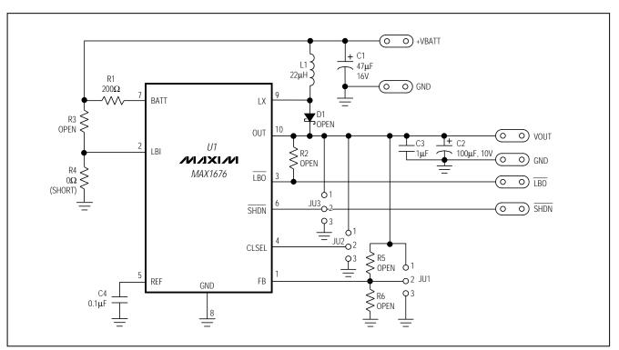
Figure 1. MAX1676 EV Kit Schematic
