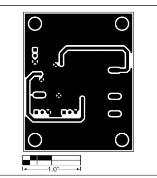
Figure 4. MAX1676 EV Kit PC Board Layout—Solder Side
