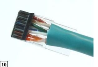
Slide the load bar down until it touches the wire separator. Trim off the excess wire in front of the load bar. It is acceptable to leave a small amount of wire showing.
