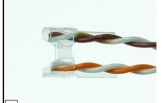
Insert the orange and brown pairs into the wire separator.
