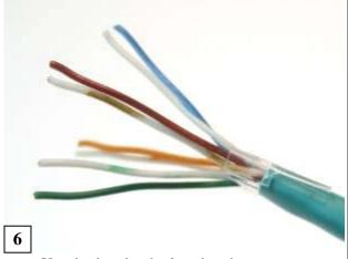
Untwist the wires back to the wire separator.
