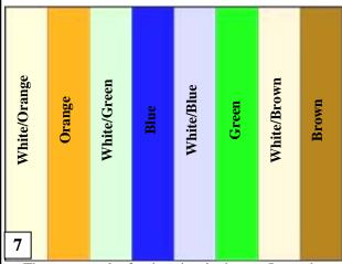
The proper order for the wires is shown. It may be necessary to add a half-twist to a pair to get the correct alignment. The twists must be as tight as possible.
