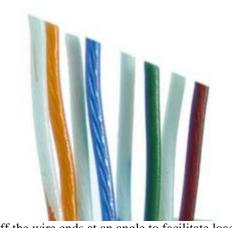
Trim off the wire ends at an angle to facilitate loading the wires into the load bar.
