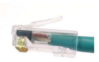
FOR A PLUG <u>WITHOUT</u> OPTIONAL STRAIN RELIEF: Insert the assembly into the housing. Terminate the plug in a standard unshielded plug crimp tool.
