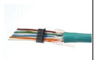
Insert the wires into the load bar.
