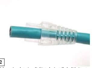
If the optional strain relief is to be installed, slide it onto the cable now.
