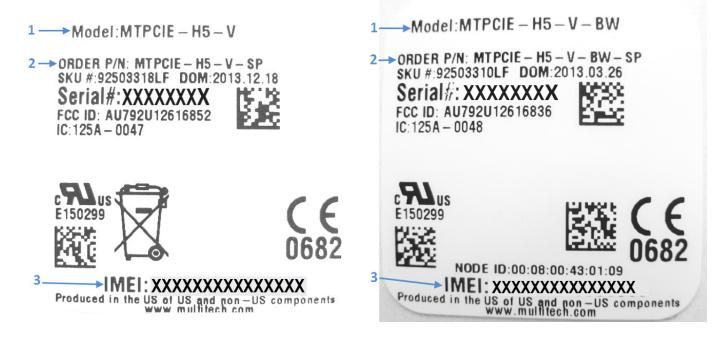
Labels are positioned on the device as follows:
