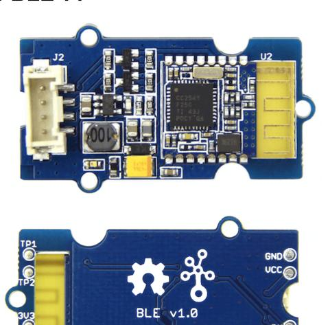
Grove - BLE v1 (Grove - Bluetooth Low Energy v1) uses a Low Energy Bluetooth module -- **HM-11**, based on TI CC2540 chip, which has AT command support. As a Grove product it's convenient to use Grove - BLE with Arduino board via Base Shield.
