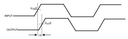
Figure 7. Input–Output Propagation Delay
