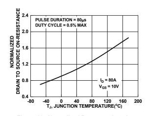
Figure 12. Normalized R<sub>DSON</sub> vs. Junction Temperature
