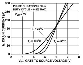
Figure 7. Transfer Characteristics
