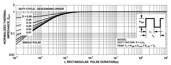
Figure 3. Normalized Maximum Transient Thermal Impedance
