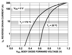
Figure 8. Forward Diode Characteristics
