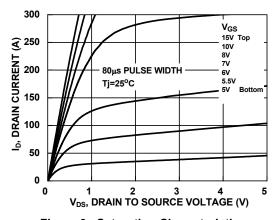
Figure 9. Saturation Characteristics
