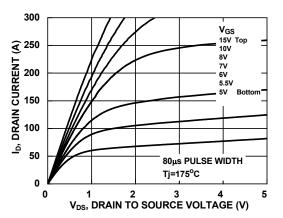
Figure 10. Saturation Characteristics
