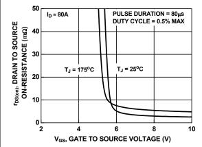
Figure 11. R<sub>DSON</sub> vs. Gate Voltage
